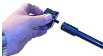
Mounting a grinding cone on the shaft
